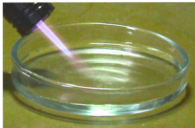
Fig. 3 Burning test, EC/GBL, 1:1, 1.5 M \text{LiBF}_4 electrolyte under laboratory gas burner
