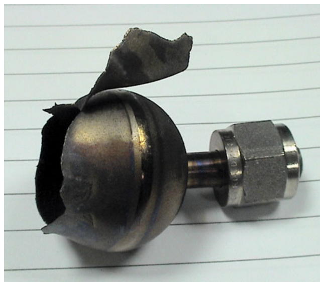
Fig. 5 Ti-bomb after ARC test with EC/EMC, 1:2, 1 M LiPF 6 electrolyte
